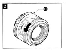
of the arrow until it stops, and release the auto extension ring from the lens.(Fig2)
